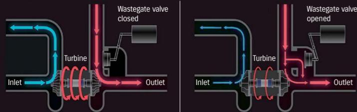
Closed for normal driving, it helps apply higher boost pressure to achieve excellent torque response.
