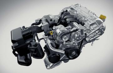
The K12N engine is well known for its uncomplicated design and easy access to maintenance items such as spark plugs, engine oil and filters.
